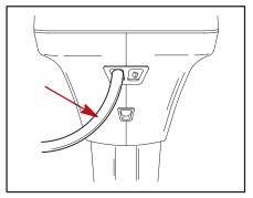
2. Attach a water hose to the fitting. Turn water on and flush for 3 to 5 minutes.
