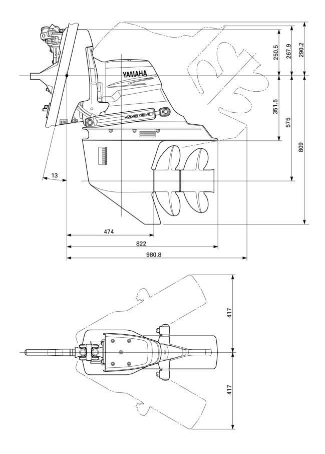
$\ast\,$  Dimensions are based on a boat transom angle of 13 °. Dimensions will change slightly when used on boats with transom angles other then 13 °.
