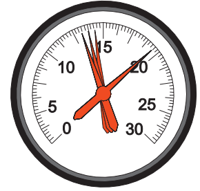
7. STICKING VALVE(S) Normally steady. Intermittently flicks downward about 4 in. Hg. from highest level.
