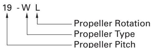
The propeller size indicates the propeller diameter, pitch and type or style.
